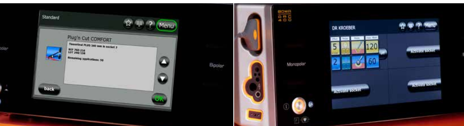
Plug'n Cut COMFORT: The COMFORT SYSTEM automatically recognises the COMFORT instrument, indicates how many times it may still be used and selects the correct parameters for the procedure.
